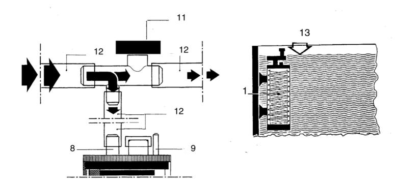
Before using the **reactor**, the rest of the  $CO_2$  system has to be assembled: The pressure regulator **regular** has to be mounted on the pressure bottle **station**. As soon as the regulator and the reactor have been mounted, the reactor can be adjusted:
